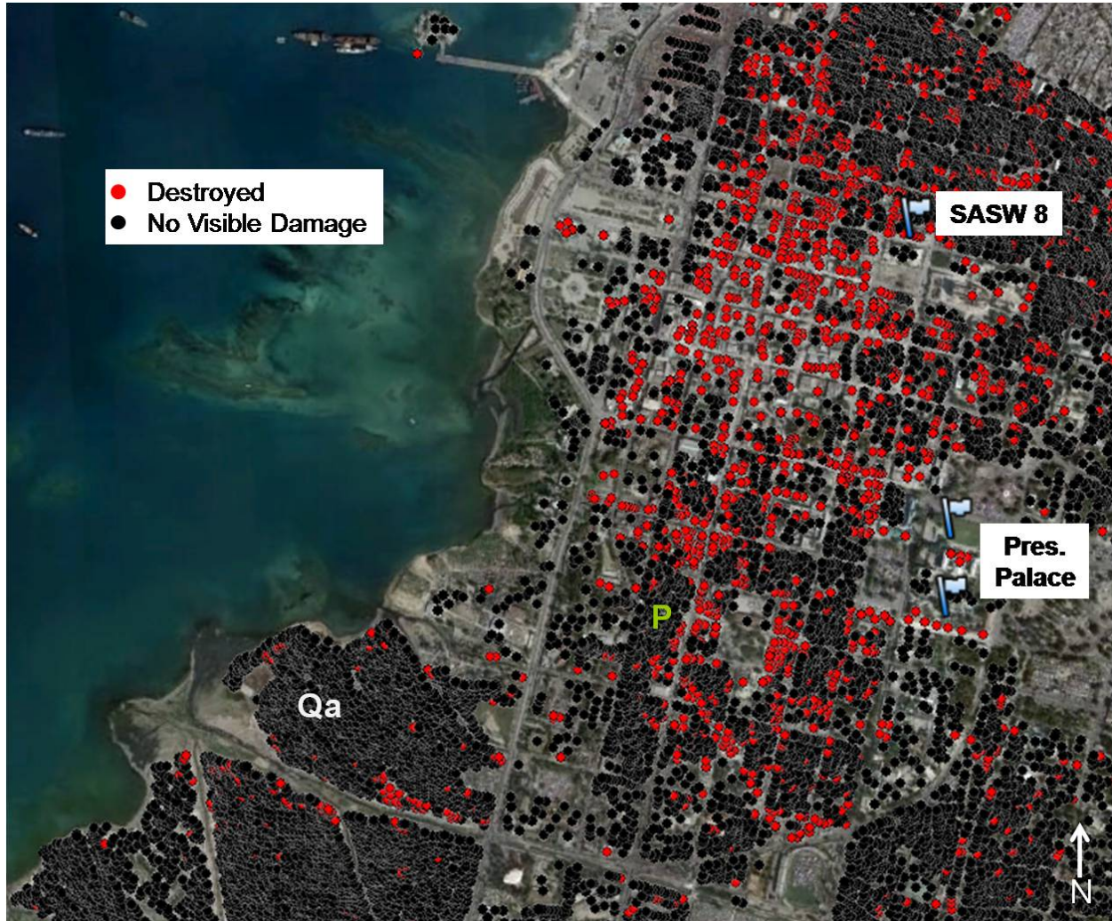
Figure 5.7 Buildings classified as No Visible Damage and Destroyed in the UNOSAT survey for the boxed area specified in Figure 5.6. Notice the heavily damaged zone lying on P deposits to the north and west of the Presidential Palace and the lightly damaged zone lying on Qa deposits in the lower left-hand corner. Most of the buildings in the heavily damaged zone were larger, multi-story, reinforced concrete structures, while most of the buildings in the lightly damaged area were smaller, densely spaced Shanty's with tin roofs (refer to the text for more detail).
